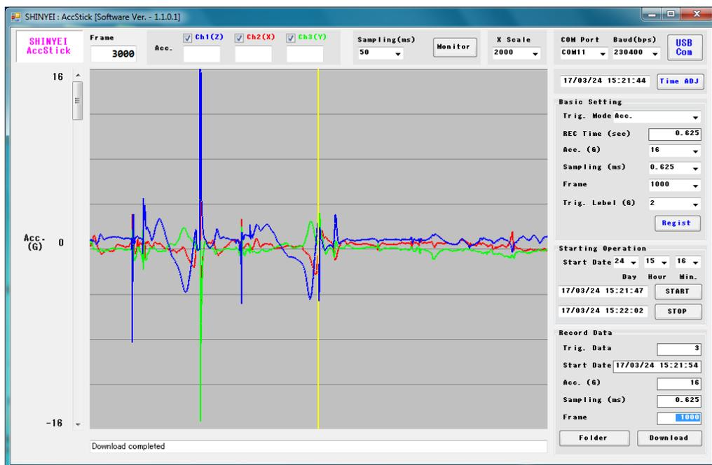
Sample shot of waveform during “Acc.” trigger mode
